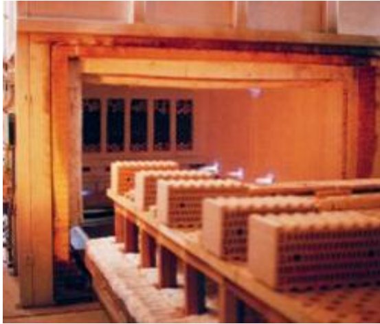
firing of original sized bricks under industrial conditions
