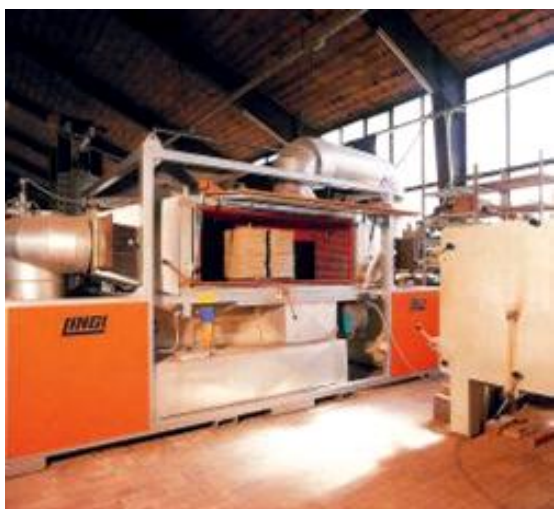
laboratory dryer for optimization of drying curves of original sized bricks
